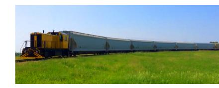
The RX500 is the only completely new locomotive designed exclusively for the industrial switching market. It incorporates the first major redesign of the industrial locomotive since diesel replaced steam. The RX500 with up to 50,000 lbs of tractive effort, is the tractive equivalent of the EMD SW1200.
